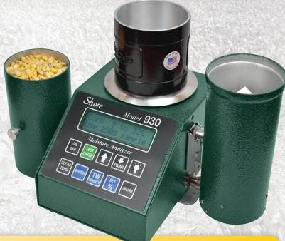
The Shore Model 930 Moisture Tester delivers quick, accurate results when testing a multitude of commodities. Featuring an integrated scale and moisture tester, the Model 930 helps verify moisture content of grain before going to market, without the need for moisture or temperature conversion tables.
